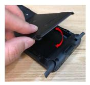
3. Press the battery cover down to secure in place. Ensure no gap existing between the device and battery cover.
